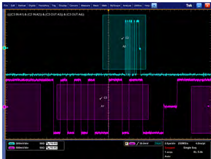
Multiple channel triggering. Visual Trigger areas can be associated with events spanning multiple channels such as packets transmitted on two USB2.0 buses simultaneously.
