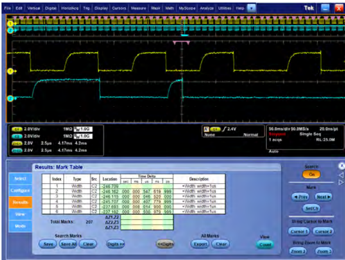
Search step 2: Wave Inspector automatically searches through the record and marks each event with a solid colored triangle. You can then use the Previous and Next buttons to jump from one event to the next.
