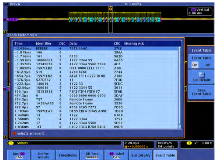
Event table showing decoded identifier, DLC, DATA, and CRC for every CAN packet in a long acquisition.
