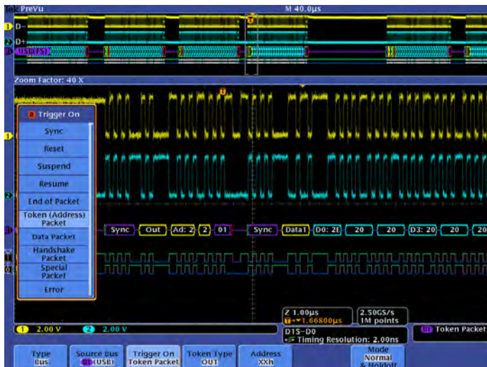
Triggering on a specific OUT Token packet on a USB full-speed serial bus. The yellow waveform is the D+ and the blue waveform is the D-. A bus waveform provides decoded packet content including Start, Sync, PID, Address, End Point, CRC, Data values, and Stop.
