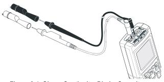
Figure 2-4. Ohms, Continuity, Diode, Capacitance Measurement Setup
