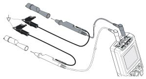
Figure 9-2. Grounding with Short Ground Lead
