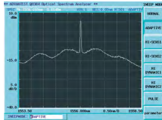
FIG. 12 Sample loop test measurement with the externally synchronized sweep function (5000 km transmission line)
