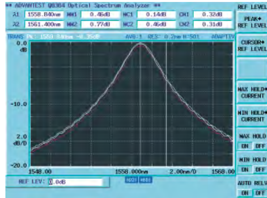
FIG. 21 MAX/MIN/CURRENT simultaneous display Display example of the characteristics when the temperature of the Band Pass Filter changes.
