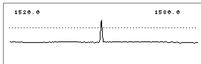
PRBS modulation graph showing raised noise floor.
