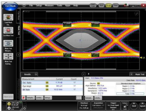
Fast transmitter characterization using eye diagram analysis and automated mask margin measurements
