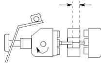
Tighten the screw to hold the electrode.
