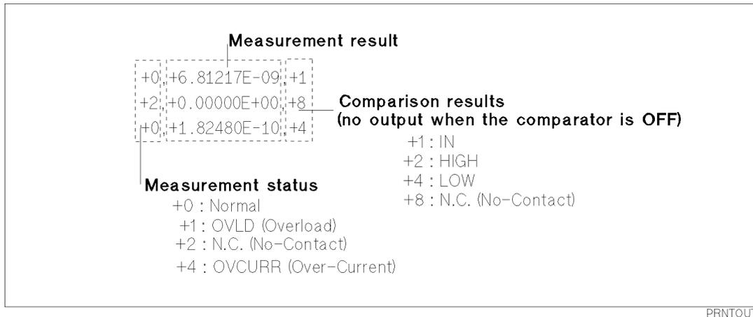
Figure 2-1. Printer Output
