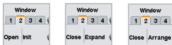
Fig. 4-25: Windows menu, softkeys for controlling the windows
