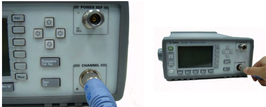
Figure 1-2 Connecting a sensor cable to power meter
