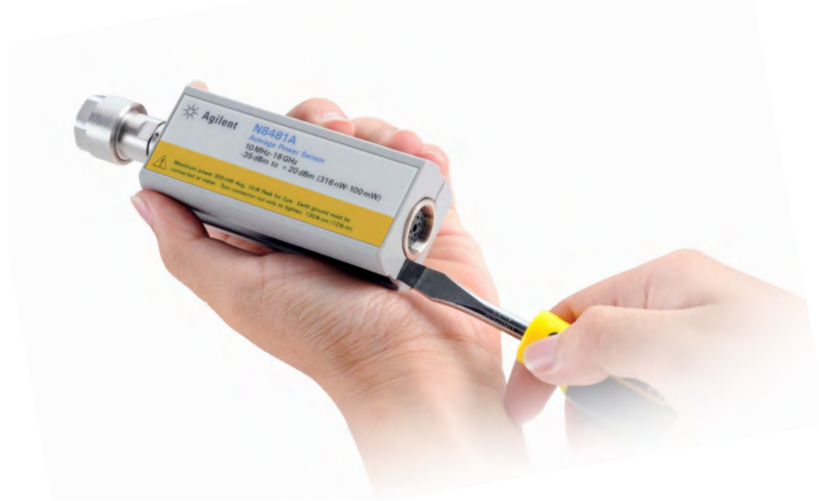
Figure 3-2 Removing power sensor shell
