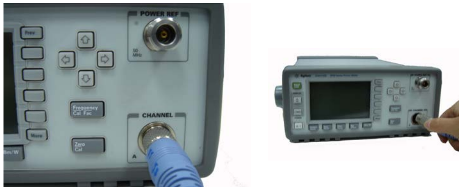
Figure 1-2 Connecting a sensor cable to power meter
