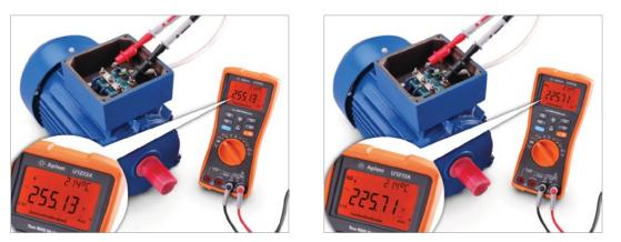
Figure 1. Comparison of voltage output from industrial motor VFD without and with Low Pass Filter functionality.
