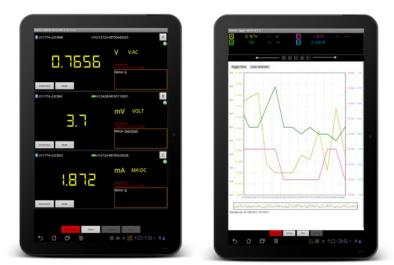
Once connected to any HH DMM via Bluetooth adapter you are able to log and view measurements graphically from smart phones and tablets.
