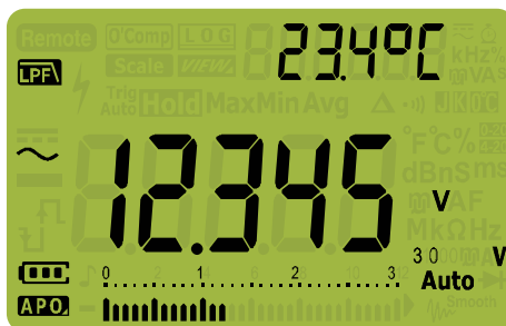
Figure 2-3 AC voltage with LPF display
