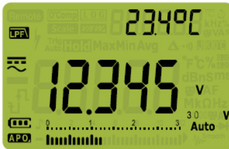
Figure 2-8 Low Pass Filter(LPF) for AC+DC voltage measurements
