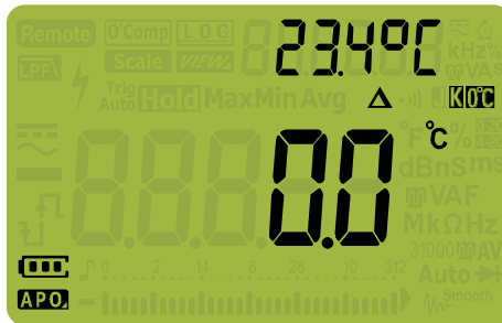
Figure 2-29 Temperature measurement without ambient compensation
