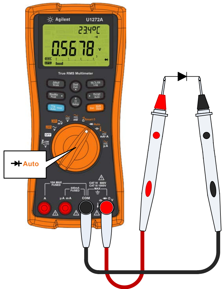
Figure 2-21 Testing forward bias diode
