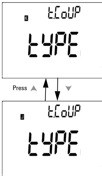
Figure 4-3 Thermocouple type setup
