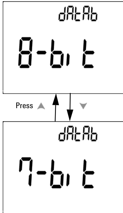
Figure 4-13 Data bit setup for remote control
