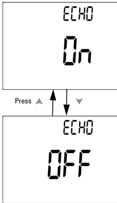
Figure 4-14 Echo mode setup for remote control
