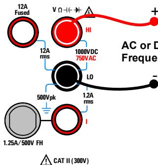
AC or DC Voltage Capacitance, Continuity Diode Test
