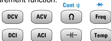
The continuity and diode test functions are shifted (shown in blue). For example, to select continuity, press:
