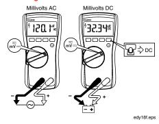
With the function switch in the  $\sqrt[m]{v}$  position, the Meter measures ac plus dc millivolts. Press \_\_\_\_\_ to switch the Meter to dc millivolts.
