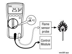
To measure flame rectification circuits:
