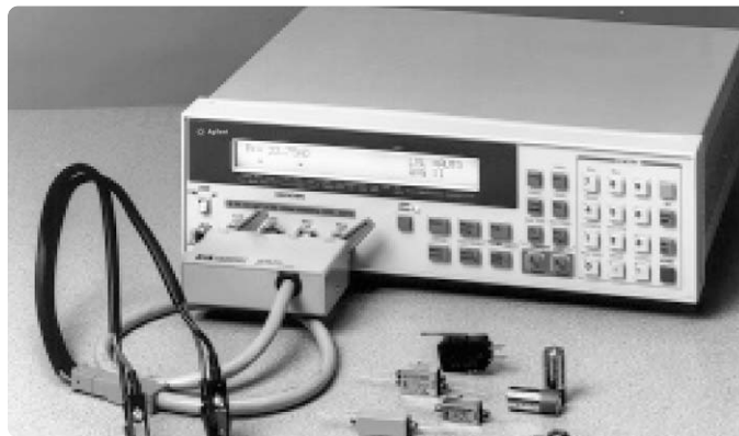
Use the milliohm meter for electromechanical contact testing.
