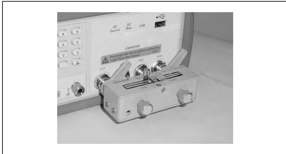
Figure 7-19 Connecting a shorting bar
