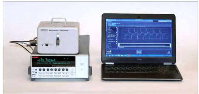
ASTM-D257-compliant High Resistivity Test System with the 6517B Electrometer, 8009 Resistivity Test Fixture, and the KickStart High Resistivity Measurement Application.
