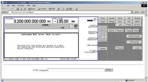
This web page remotely accesses all signal generator functions and operations. Use the mouse pointer to click on the signal generator's hardkeys and softkeys. The results of each mouse click selection will be displayed on the web page. For example, click on the Frequency hardkey then use the front-panel key pad to enter a frequency. You can also use the up and down arrow keys to increase or decrease the frequency.
