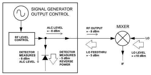
The internally leveled signal generator RF output (and ALC level) is -8 dBm. The mixer is driven with an LO of +10 dBm and has an LO-to-RF isolation of 15 dB. The resulting LO feedthrough of -5 dBm enters the signal generator's RF output connector and arrives at the internal detector.
