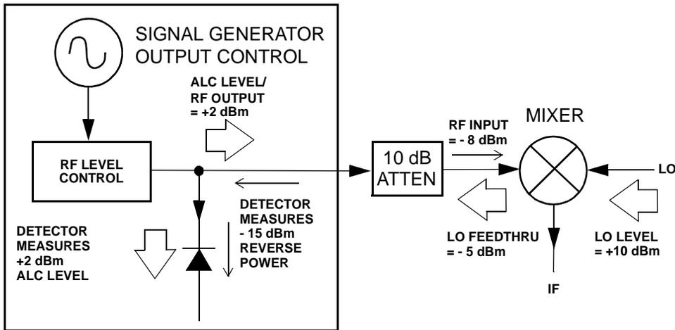
Compared to the original configuration, the ALC level is 10 dB higher while the attenuator reduces the LO feedthrough (and the RF output of the signal generator) by 10 dB. Using the attenuated configuration, the detector is exposed to a +2 dBm desired signal versus the -15 dBm undesired LO feedthrough. This 17 dB difference between desired and undesired energy results in a maximum 0.1 dB shift in the signal generator's RF output level.
