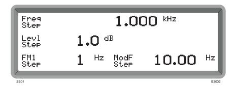
Fig. 4-7 Step setting display showing default settings
