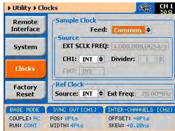
Figure 3-16: Modifying the SCLK and 10MHz Clock Source
