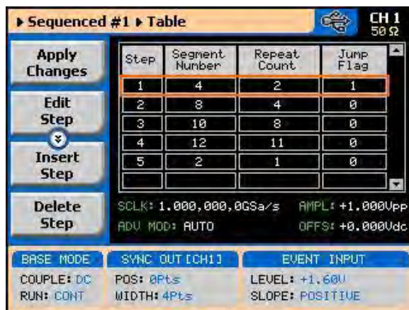
Figure 1-11: Typical Display of a Sequence Table
