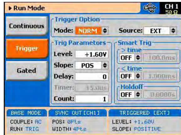
Figure 3-10: Trigger Run Mode Parameters
