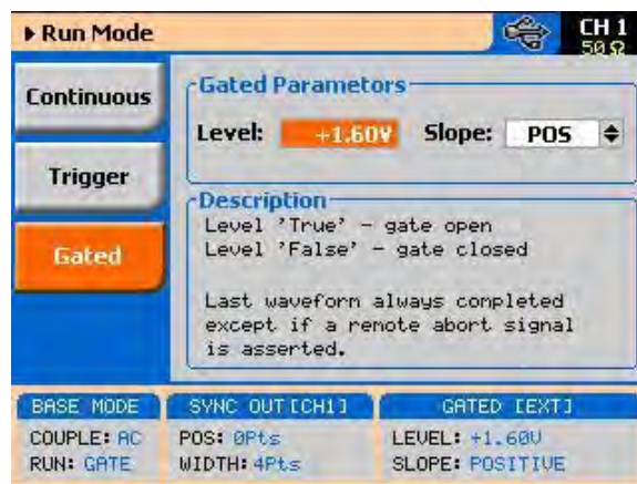
Figure 3-11: Gated Run Mode Parameters
