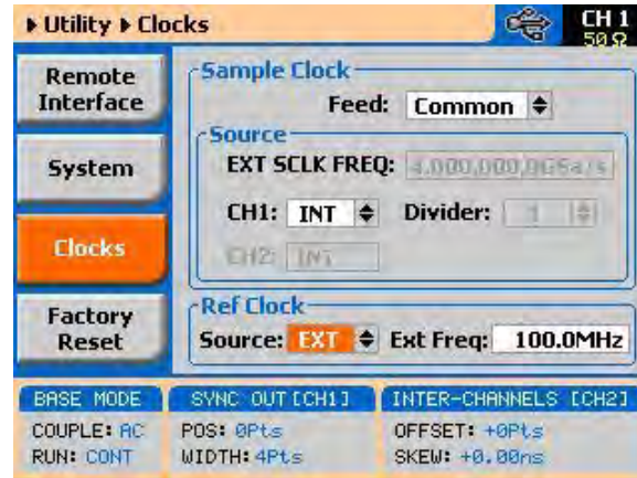
Figure 3-18: Using an External Sample Clock Example
