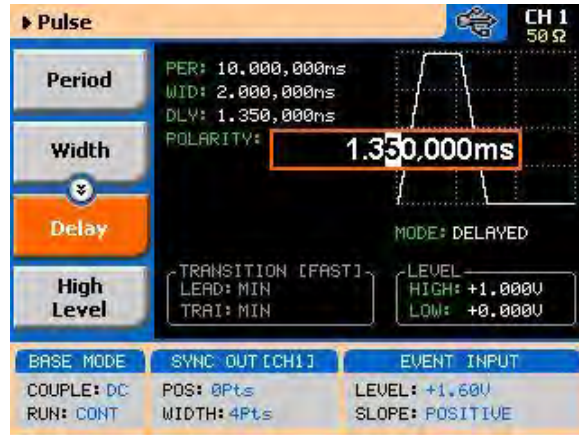
Figure 3-45: Programming the Single Pulse Delay Parameter
