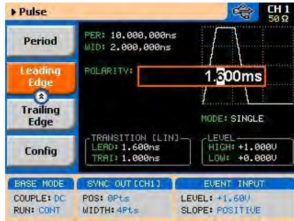
Figure 3-52: Leading Edge Programming Example
