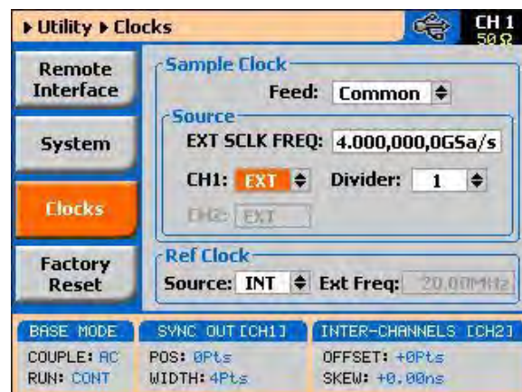
Figure 3-17: Using an External Sample Clock Example
