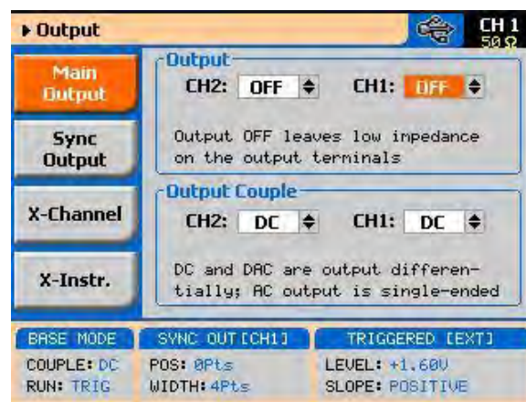
Figure 3-6: Selecting an Output Couple Path
