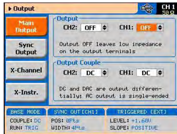
Figure 3-3: Enabling and Disabling the Outputs
