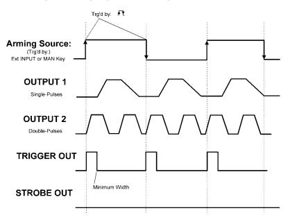
NOTE The PLL cannot be selected as the arming source. Select continuous pulses mode with the PLL as PERIOD SOURCE to achieve the same result.
