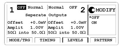
When you press SHIFT + MORE (GRAPH) or the LEVELS softkey, you will see a graphical representation of the level parameters. The currently selected parameter is displayed in the Modify/Enter area and is indicated in the graphical display.
