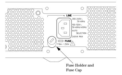
**3** Replace the fuse with the equivalent part
