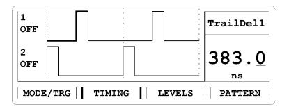
The trailing delay is the absolute delay from the start of the pulse period to the start of the trailing edge. In this format the trailing edge remains fixed relative to the start of the pulse period if you adjust the pulse-delay (leading-edge delay) or the pulse period.
