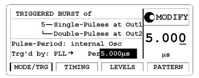
To set the **timing parameters** as required:
