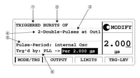
In this screen, you can set up the signal to be triggered or continuous, and to be a pulse stream or a burst (several pulses followed by a pause) consisting of single or double pulses. Furthermore, you can specify the pulse and trigger sources.
