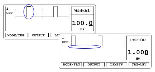
Use the left/right cursor keys to toggle between the individual timing parameters.
