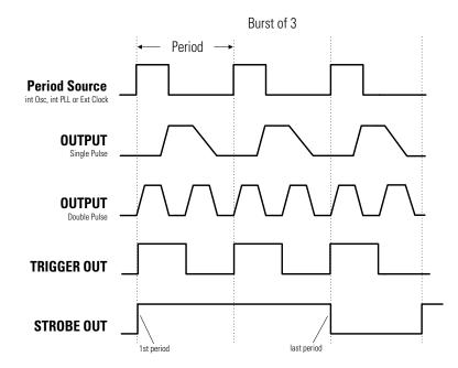
**Characteristics** • A burst of pulse periods is repeated continuously.
