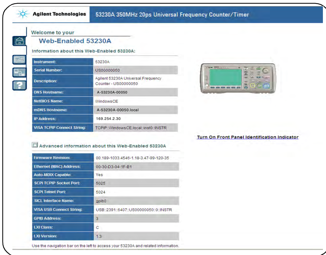
Figure 2-1. The 53230A Web-Enabled Interface ‘Welcome Page’.
