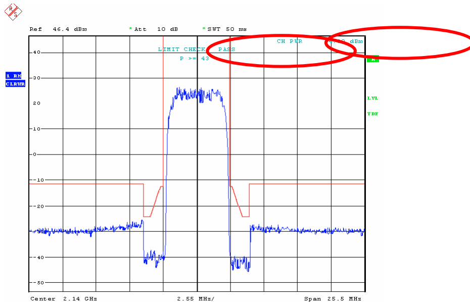
Fig. 4-33 Measurement of the spectrum emission mask
