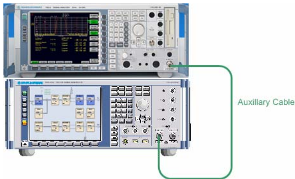
Fig. 3-3 Test setup during normalization
