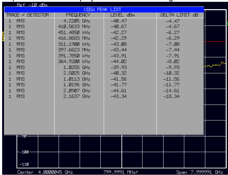
Fig. 4-56 Display of the peak list for spurious emissions
