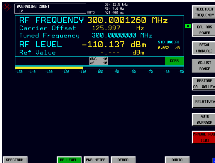
Fig.2-8 Tuned RF Level measurement with Averaging
