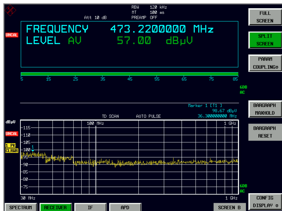
Fig. 4.16 Typical split-screen display
