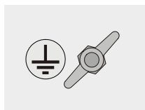
Grounding conductor connection
