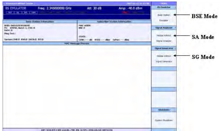
Figure 9 E6651A Test Set Operational Mode Selection Window
