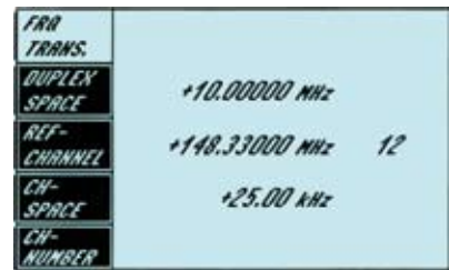
Channel numbers and duplex spacing can be defined and used instead of frequencies
