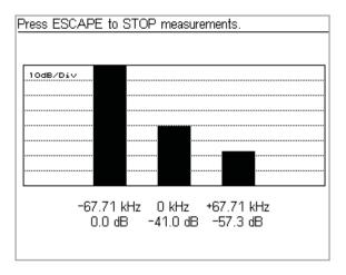
The large dynamic range of 60 dB for I/Q alignment allow for optimal tuning of phones. The bar graphs are clearly visible and the numbers provide accurate results.
