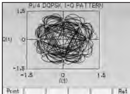
IQ Constellation display allows for comprehensive digital modulation testing
