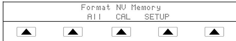
Use Format NV Memory (non-volatile) with caution. Changes are non-reversible. The softkeys function only when the rear-panel CALIBRATION switch is set to ENABLE, except for the softkey SETUP, which is not dependent on the CALIBRATION switch position.
