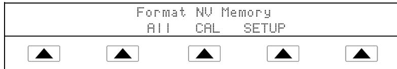
All the softkeys in this menu require the rear panel CALIBRATION switch to be in the ENABLE position. The nonvolatile memory contains calibration constants and dates, setup parameters, and the user report string. In the case of calibration constants, factory defaults are the same for all Calibrators. They are not the calibration constants obtained when the 5820A was calibrated by the factory before shipment. The softkeys are:
