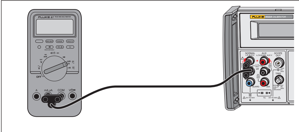
Figure 4-19. Cable Connections for Testing an 80 Series Current Function
