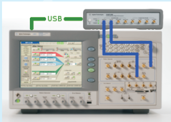
Agilent N4916B De-Emphasis Signal Converter connected to N4903B Serial BERT
