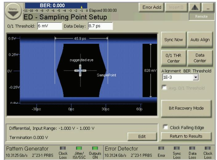
Figure 11. Auto alignment (center) simplifies correct sampling
