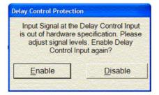
You can enable the input after reducing the voltage to safe level.
