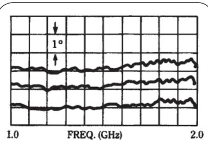
Center trace is phase response of 8491A -6 dB attenuator from 1.0 to 2.0 GHz taken with Agilent 8410 network analyzer. Top and bottom traces are  $\pm 1^\circ$  calibration. Linear phase component has been compensated for with a line stretcher. Response, therefore, shows nonlinear phase deviation of  $< \pm \frac{1}{2}^\circ$  over 1 to 2 GHz band.
