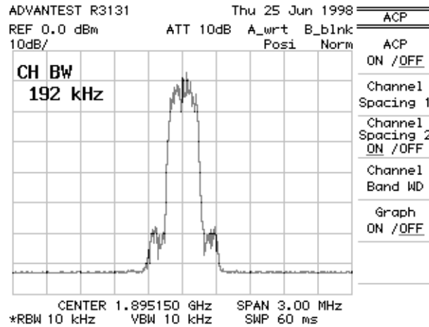
Figure 2-61 Setting the Specified Bandwidth
