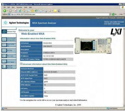
At the left side of the page are a set of tabs that provide access to configurati on informatio n for the instrument, plus the ability to control it through the web interface.
