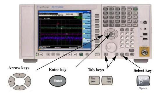
The following keys are used in the initialization process:
