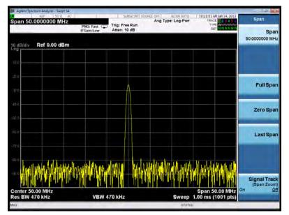
The 50 MHz reference signal appears on the display.
