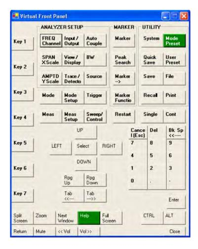
When you click a button in the Virtual Front Panel, it performs the operation of the corresponding instrument front-panel key. The buttons at the left of the panel, named Key 1 through Key 7, perform the operation of the respective softkeys. The Rpg Up and Rpg Down keys perform the operation of the knob.
