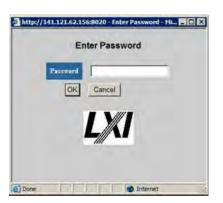
By default, this password is set at the factory as "agilent". However, you may subsequently change the password. (Press **System**, **I/O** Config, **Reset Web Password** on the instrument front panel to change the password.)
