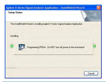
**NOTE** The installation process can take up to 45 minutes. Do not turn the instrument power off or serious damage may occur. If any pop up windows appear, click **OK** or **Ignore** to proceed.
