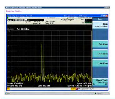
2. Click **Display Front Panel Keys**. This brings up a virtual keyboard that can be used to control the instrument.
