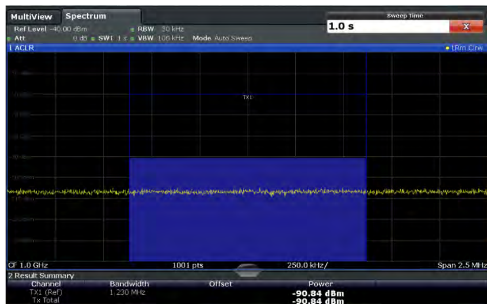
Fig. 5-33: Measurement of the R&S FSW's intrinsic noise power in a 1.23 MHz channel bandwidth.
