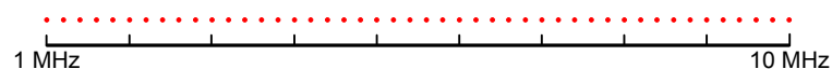
Fig. 6-21: Linear x-axis scaling: the distance between the sweep points is equal, e.g. 200 kHz
