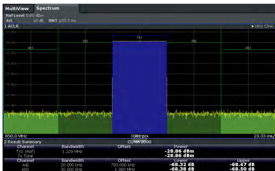
Fig. 5-21: Measuring the channel power and adjacent channel power ratio for CDMA2000 signals with zero span (Fast ACLR)
