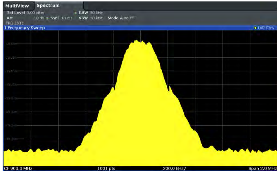
Fig. 6-30: GSM signal with GATE OFF
