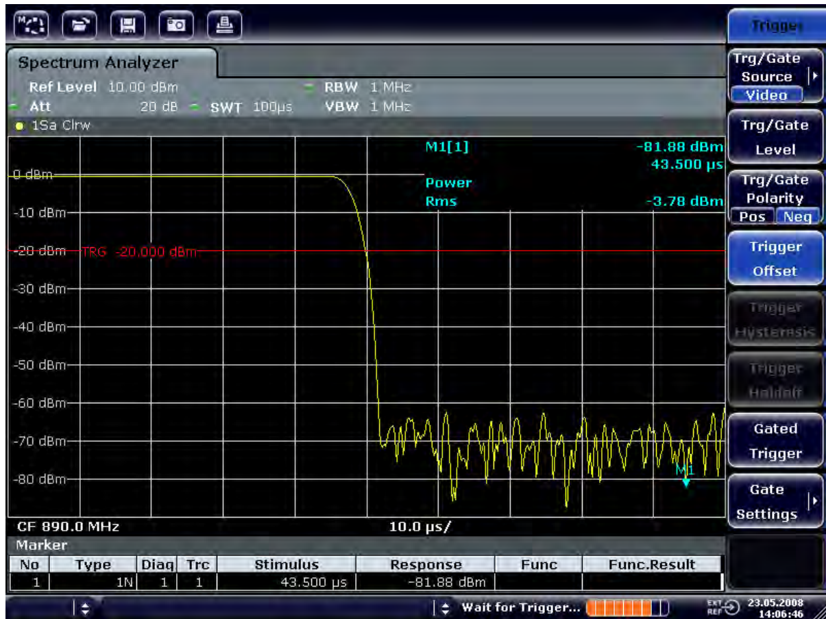
Fig. 6-10: Falling edge of the GSM burst displayed with high time resolution
