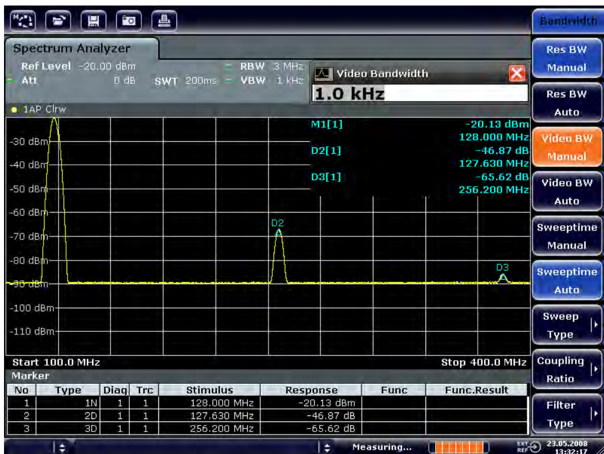
Fig. 6-3: Suppression of noise during harmonics measurement by reducing video bandwidth
