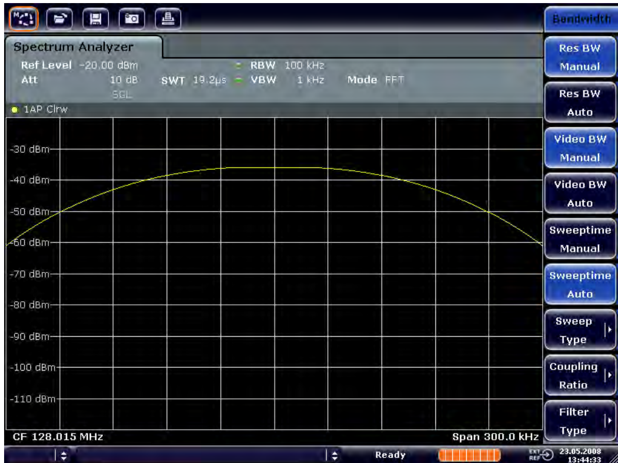
Fig. 6-5: Measurement of two equally-leveled RF sinusoidal signals with a resolution bandwidth which is larger than their frequency spacing
