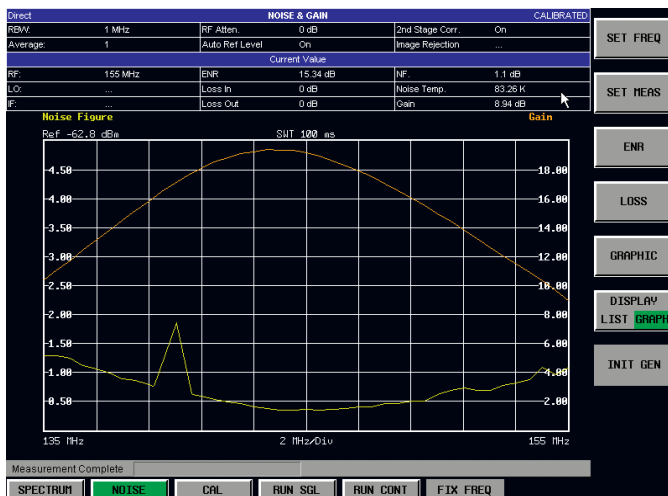
Noise figure measurement with the R&S®FS-K30 option.
