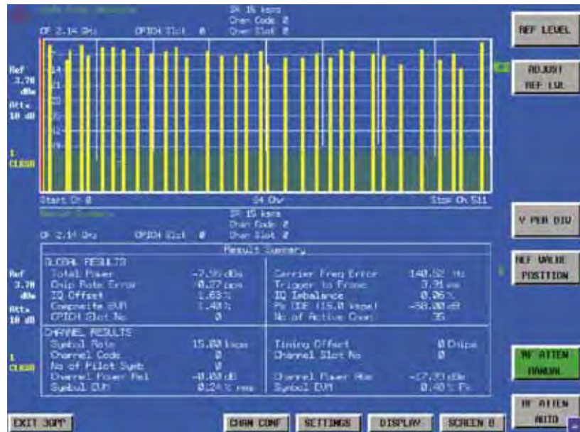
WCDMA code domain power measurement with the R&S® FSQ and R&S® FS-K72.
