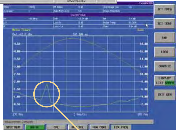
Noise figure measurement using Application Firmware R&S®FS-K30.
