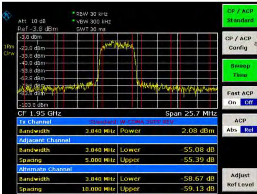
Fig. 2–24 Measuring the relative adjacent channel power on a W–CDMA uplink signal
